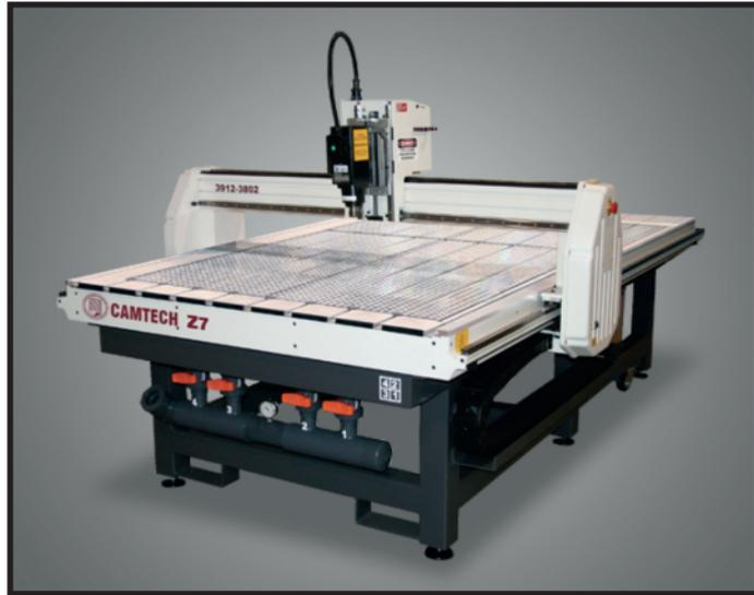
**SLP (UK) Ltd's** recent purchase of a CNC Router means that we are now able to offer a precision cutting / machining service to satisfy all your needs in house! At SLP (UK) Ltd our CNC Router ensures repeatable and reliable accuracy with an edge finish to our plastic sheet that is of the highest quality. We can cut panels to whatever size you require from 2.45 x 1.25m master sheets providing a swift and reliable service.
